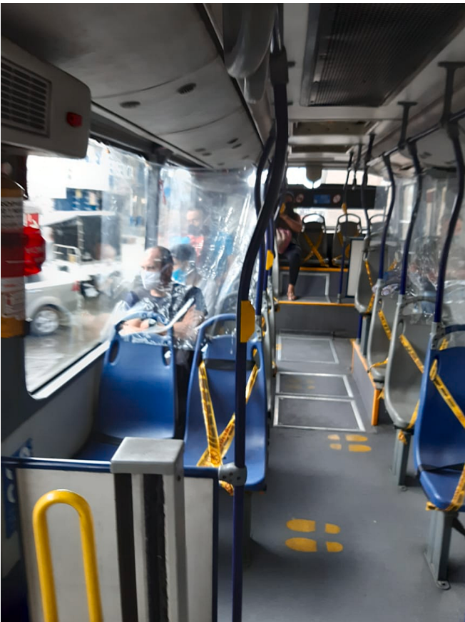
Fig. 5. Flexible partitions installed in a bus carrying users. Source: (Anonymous technician, 2020)
